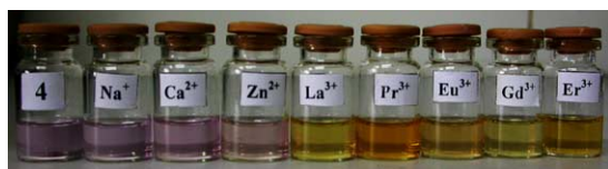
Figure 1. Color change of compound 4 (50 \mu\text{M} ) in acetonitrile induced by addition of 2 equiv of metal nitrate (from left to right: compound 4 without metal ion; addition of \text{Na}^+ ; \text{Ca}^{2+} ; \text{Zn}^{2+} ; \text{La}^{3+} ; \text{Pr}^{3+} ; \text{Eu}^{3+} ; \text{Gd}^{3+} ; \text{Er}^{3+} ).
